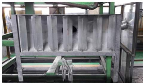
Set up Dust Collector for dust reduction
